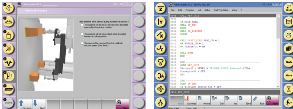
Additional screen displays of the R8 control system: QuickNew (left) and TextEditor. R8 控制系統的附加屏幕顯示：QuickNew（左）和文本編輯器。
