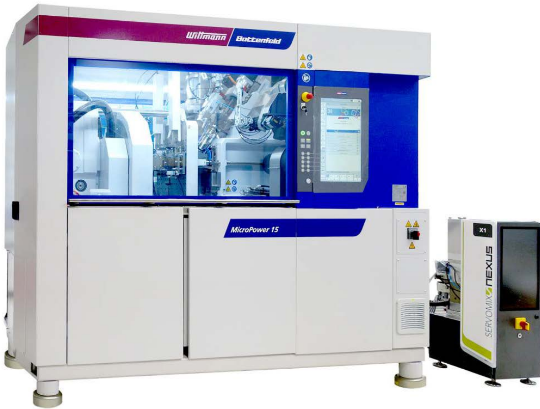
Fig. 1: MicroPower 15/10H/10H COMBIMOULD with liquid dosing unit for LSR 圖: MicroPower 15/10H/10H COMBIMOULD 帶有用於 LSR 的液體計量裝置
