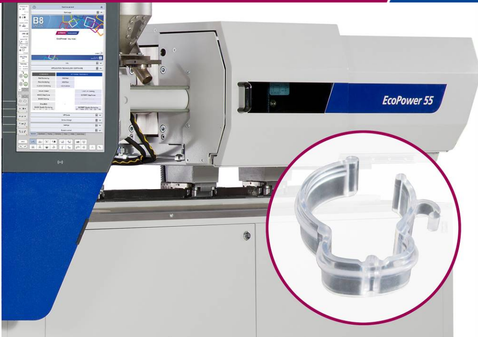
Fig. 3: hose clamp for medical technology, produced on an EcoPower 55/350 WITTMANN 4.0 production cell (photo of hose clamp: WILamed GmbH)
