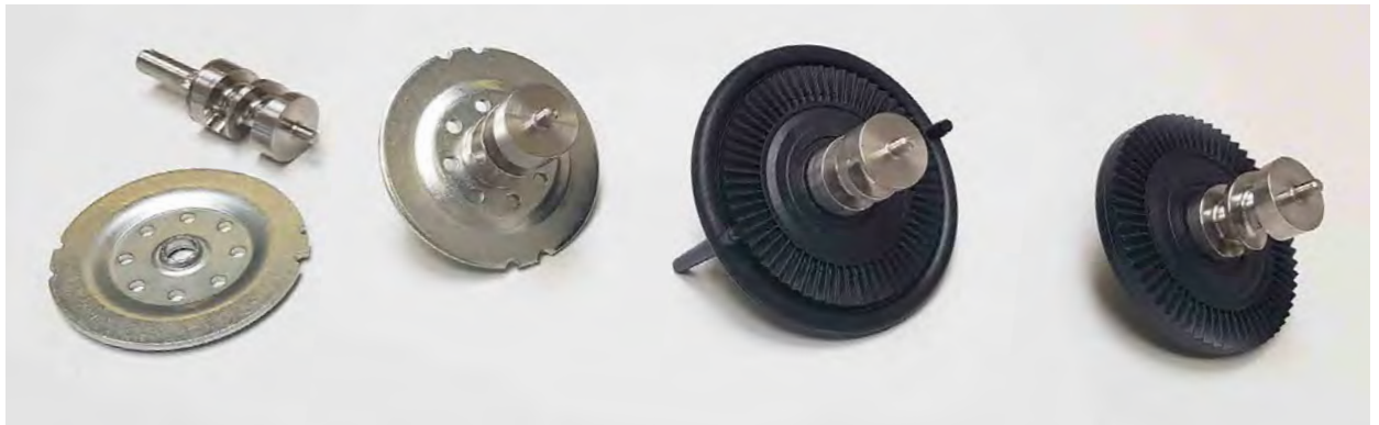
From left to right: two-part metal insert (consisting of shaft and disk), injection-molded part, finished part.
