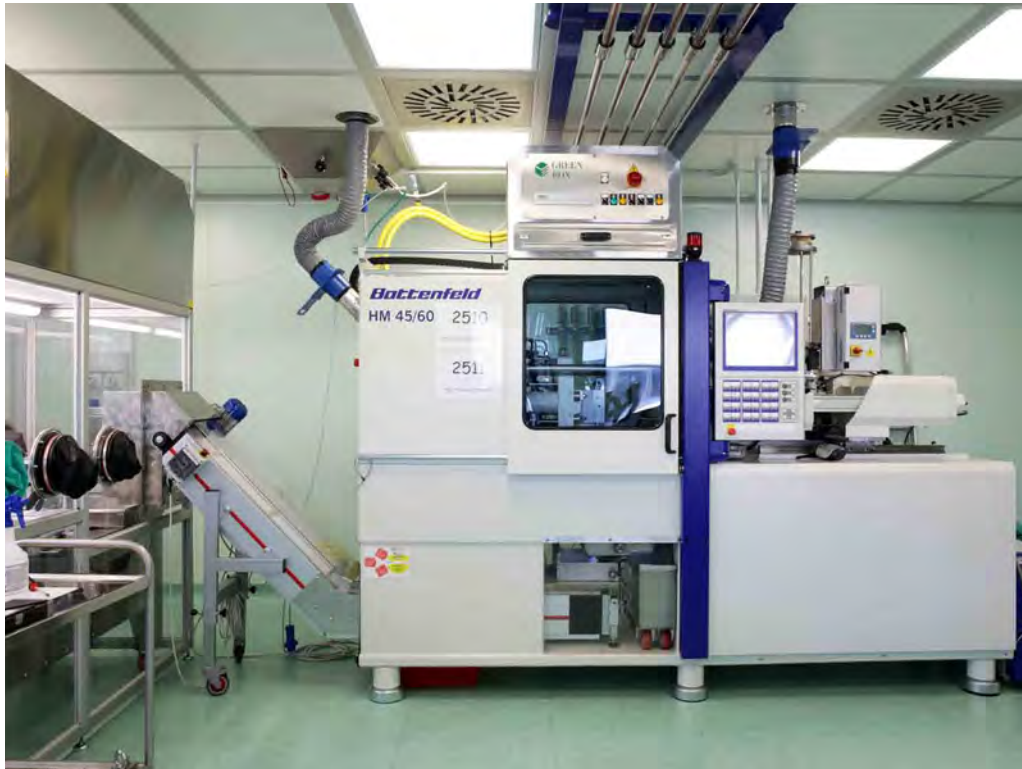
Picture left: To ensure sterility, injection molding of bio-resorbable products is carried out in an ISO class 7 clean room. In this picture: the production cell with the HM 45/60 from WITTMANN BATTENFELD.
