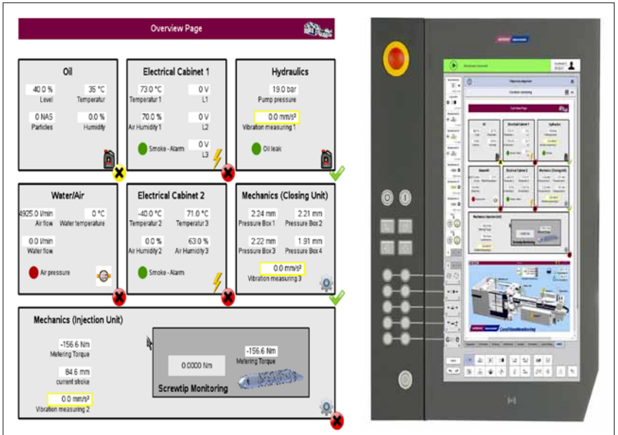
Fig. 4: Overview of condition values on the B8 machine control system.
