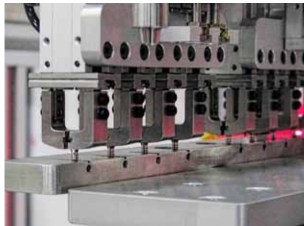
Left: Micro-inserts loaded on pins on a shuttle prior to pickup by a robot. Red light is flash illumination for camera inspection. Right: EOAT picking micro-inserts from nest.
