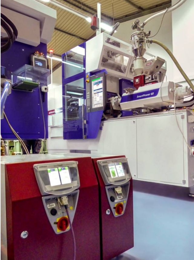
Fig. 3: WITTMANN TEMPRO plus D temperature controllers integrated in Insider cells (Photo: WITTMANN BATTENFELD)
