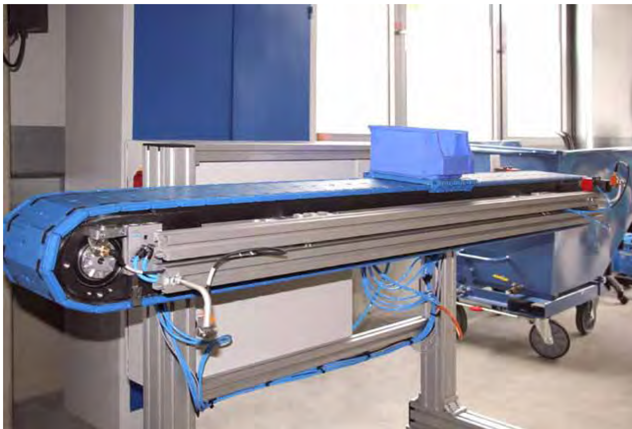
Flexi conveyor (testing appliance) from ErgoTek consisting of plastic parts made by Happ.
