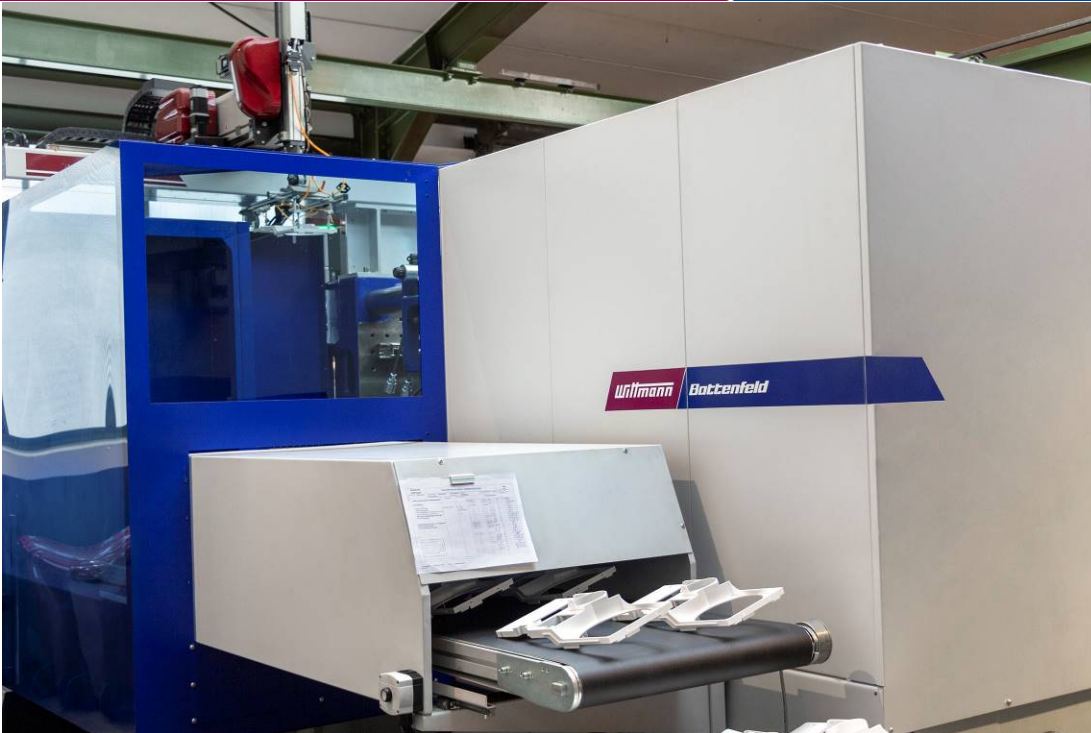
Fig. 2: Production of a housing component for a beverage dispenser with SmartPower 300/1330 with insider cell (Photo: WITTMANN BATTENFELD)
