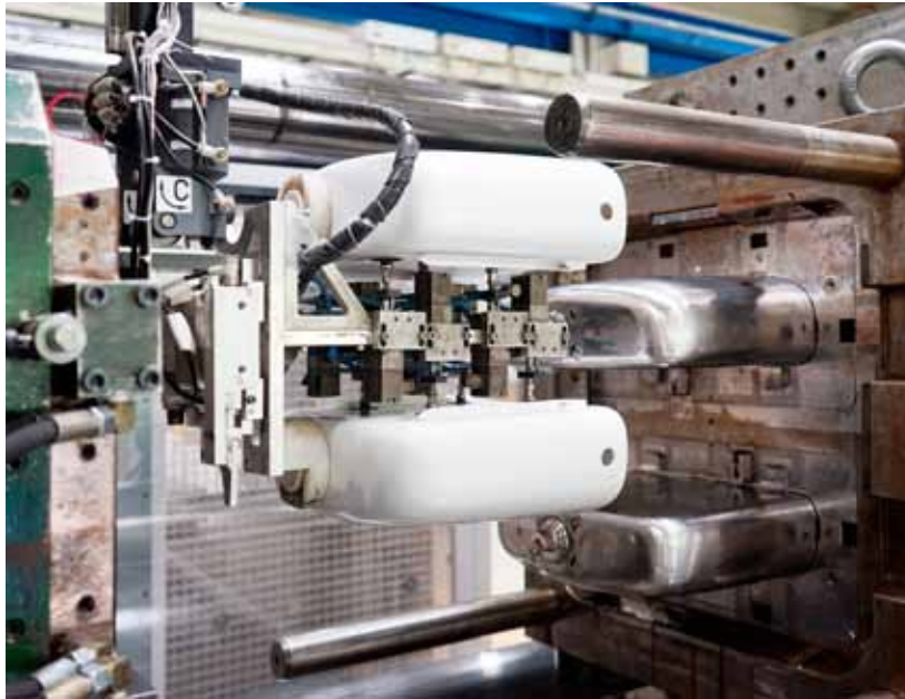
View into the mold space of the application at the moment of parts removal.
