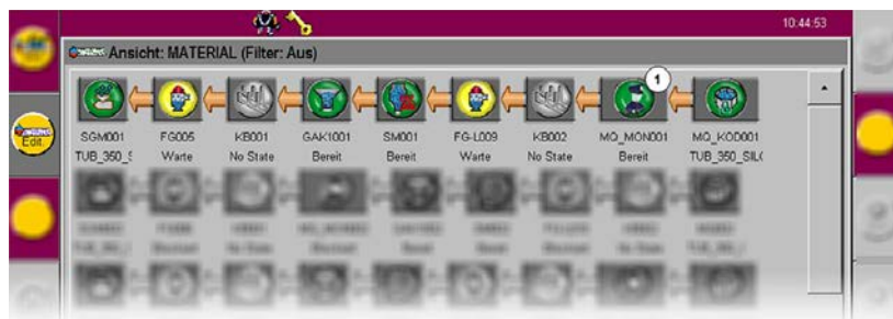
Symbols for storage place monitoring on the M7.3 IPC network control panel:
