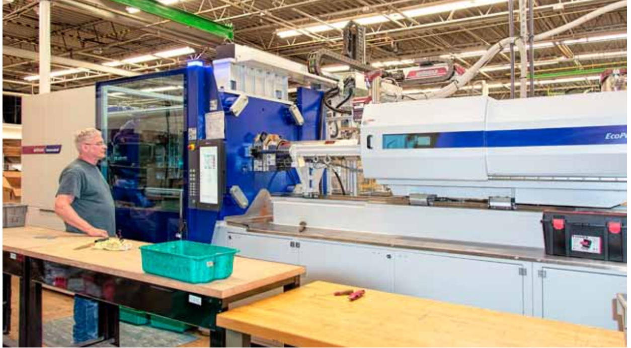
Bob Parkhurst at the B8 control of DMT's EcoPower 300 electric injection molding machine.
