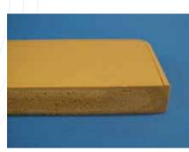
Wall thickness expanded by breathing core: 50 % lighter
