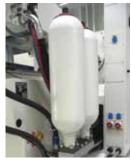
Optional hydraulic accumulator for high-speed injection
