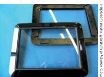
Display: insert-molded glass panel, 2 mm, with variations in wall thickness
