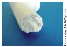
Fracture pattern of thick-walled part made of PBTGF 30, 66 % lighter
