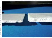
Part on the left: plate made of PS, 3.5 mm, 22 % lighter / Part on the right: breathed from 3.5 to 8.5 mm, 66 % lighter
