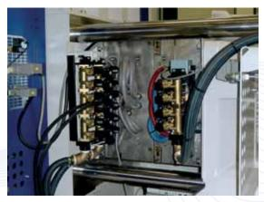
Correction of the mold temperature by addressing the individual cooling circuits of the WITTMANN WFC: Water Flow Control.
