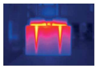
*IR* – picture of a molded part immediately after demolding.
