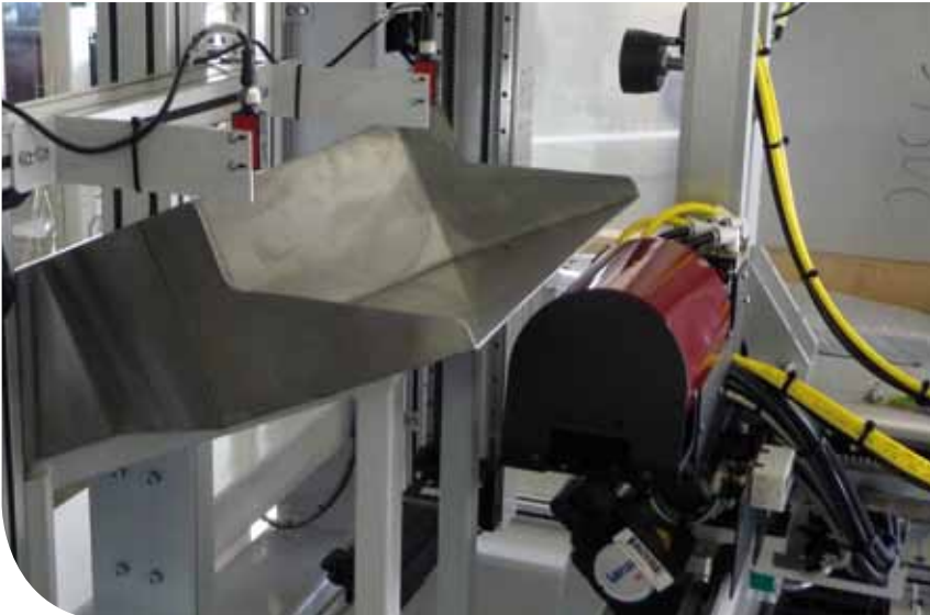
Label detection: color sensor
