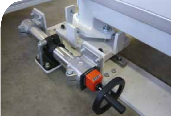
Floor guiding rail for mold thickness adjustment
