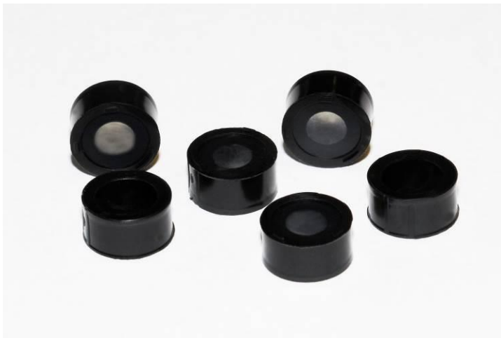
Fig. 2: Membrane made of PP and EVA9 由 PP 和 EVA9 制成的膜
